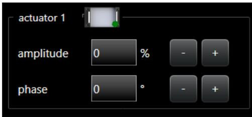
This group allows you to parametrize one actuator (the first one in this case). There is one group for each actuator of the Asycube.
