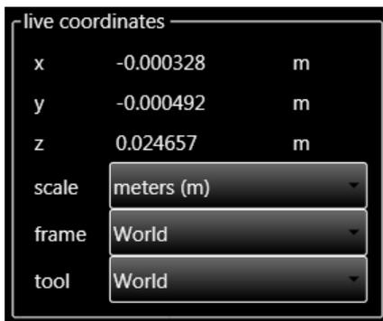
This field indicates the position of the robot in real time. By default, the position is sent in the basic reference (world: frame 0 tool 0, in meters). The dropdown lists make it possible to select which frame and which tool should be used to read the current position of the robot.
