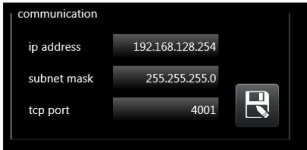
In this group, you can change IP address, subnet mask and tcpport of Asycube electronic. Click on the button to apply the modifications.
