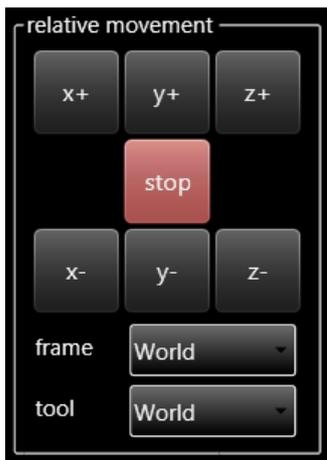
The buttons in this zone are used to move the robot relative to the current position in a given frame and using a specified tool.
