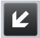
This button activates the platform vibration B which has as standard configuration to move parts forward left.
