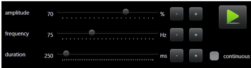
This group allows you to tune the hopper actuator and the duration of the vibration.
