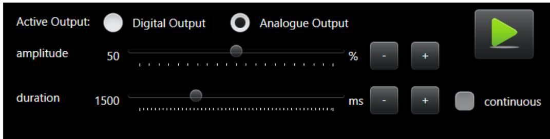
This group allows you to tune the outputs activations and the duration of the activation. It is usually used to control the external hoppers vibration.
